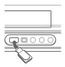
**Inserting the USB Memory Stick**Insert straight-in until it fits into place.
